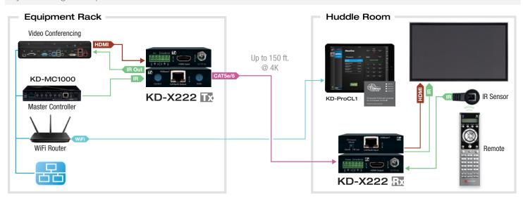
\* For all installations, we highly recommend use of KD-CAT6STP1X STP cabling, especially in hostile electrical environments. The shield of CAT6STP must be soldered on both ends to the shield of RJ45 connector used. The CAT5/5e/6 cable has to be terminated according to TIA/EIA-568-B standard. The use of STP CAT5, 5e is not recommended.
