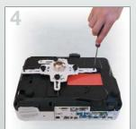
Fix the adjustable arm plate to the projector by positioning the plate's screws in correspondence to the designated holes on the bottom of the projector.
